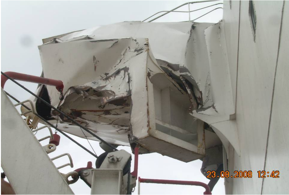
MV Yossa Bhum- Damaged portside Bridge wing
