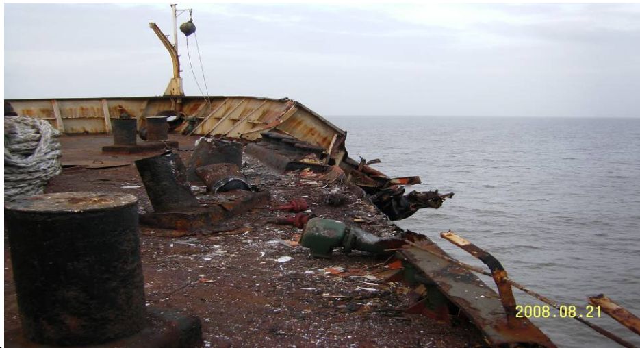
MV Surfing Jad – Damaged Forecastle deck
