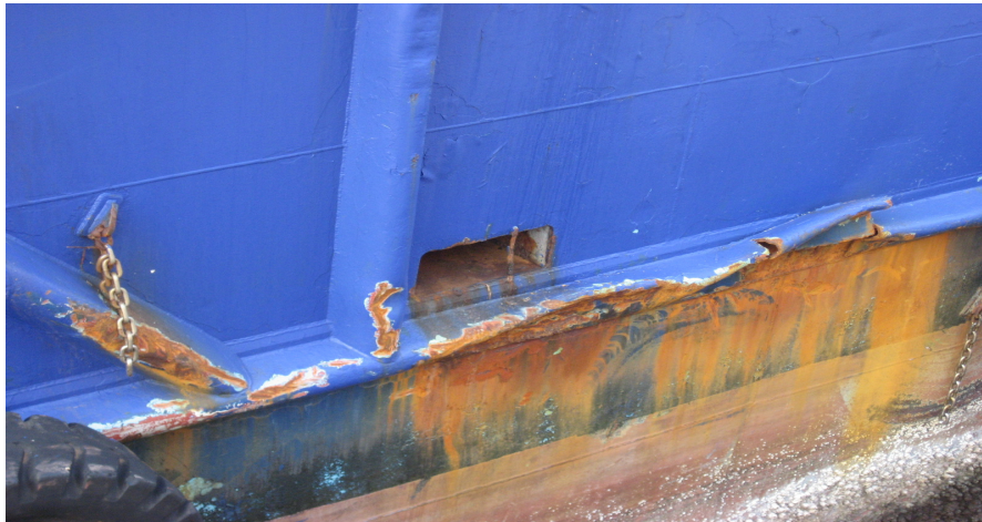
Damaged plate of C S Topper
